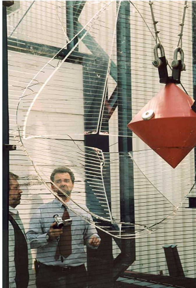
Fig. 8: Assessment of the broken specimen; all fragments are hold in place by PA-filaments
