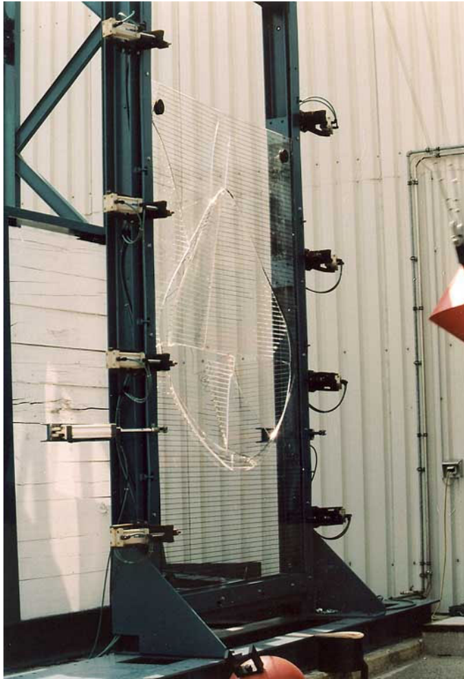
Fig. 6: Backswing of the pendulum after the first impact (photograph)
