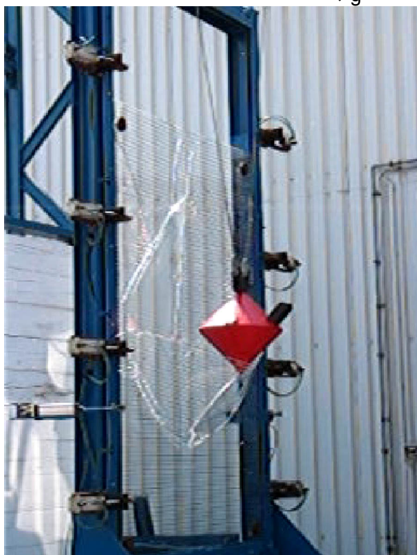
Fig. 4: Impact of the steel double-cone impactor and the backswing of the pendulum (cut off from the video film sequence e → g)
