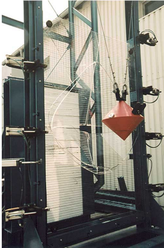
Fig. 7: Condition of the broken specimen after the impact test (no loose, large, sharp and heavy fragments were produced)
